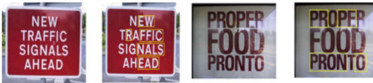
Fig. 6 Text retrieval from the input image using bilateral filter (original image and text detected)
