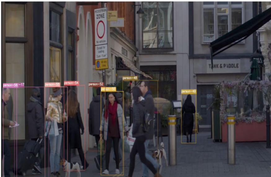
The above image is the snippet of the output showing the objects that are detected using YOLO algorithm. This output is then stored in cloud and can be used when needed.
