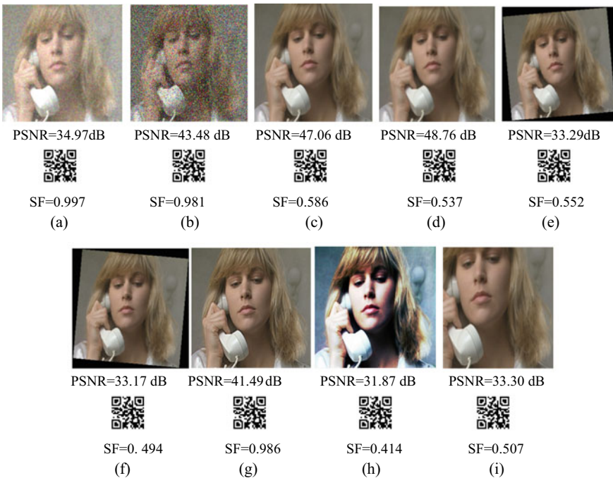
Fig. 2 Watermarked video frame with detected watermarks under a Gaussian noise, b Salt and pepper noise, c average filtering, d median filtering, e rotation in anti-clock wise direction, f rotation in clock wise direction, g sharpening, h histogram equalization, i cropping
